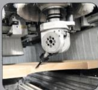
Boring on tilted surfaces.
